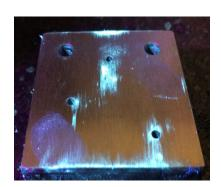
Fluorescing particulates and hydrocarbon residues on a not yet cleaned part become visible under ultraviolet light.
